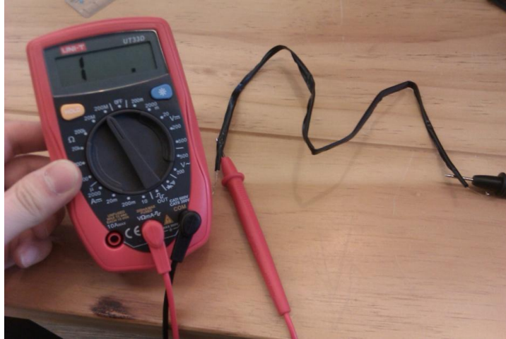
Figure 26: Resistance Exceeds 200M\Omega
