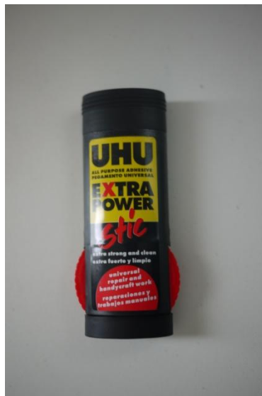
Figure 9: All Purpose Glue Used to Attach PCB and Neoprene in the Jacket
